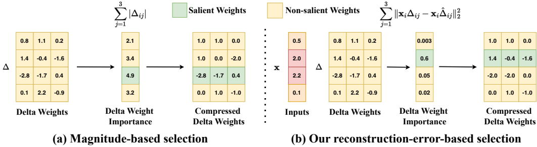
Figure 2: An illustration comparison between the magnitude-based selection of salient delta weights and our reconstruction-error-based selection method. Given a delta weight matrix \Delta \in \mathbb{R}^{m \times n} , its quantized version \hat{\Delta} , and input \mathbf{x} \in \mathbb{R}^m , where m and n denote the number of input and output channels, respectively, our method measures the importance of each input delta channel by \sum_{j=1}^n \|\mathbf{x}_i \Delta_{ij} - \mathbf{x}_i \hat{\Delta}_{ij}\|_2^2 .
