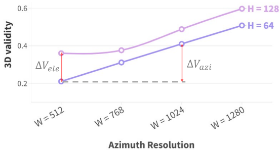
Figure 2. Statistics on SemanticKITTI [2]: 3D validity (proportion of projected points) with different azimuth ( W ) and elevation ( H ) resolutions. Comparable increases are observable when doubling azimuth and elevation resolution ( \Delta V_{azi} , \Delta V_{ele} ).
