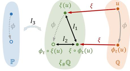
Figure 2. Illustration of our proposition. Here  $\xi$  represents the domain translator. Term  $I_1$  measures the model’s consistency loss on the domain-translated example pairs. Term  $I_2$  measures the model’s consistency loss on a ground-truth transformed example and its approximated version generated by the domain translator, which can be minimized if the domain translator is equivariant. Term  $I_3$  measures how well the push-forward distribution matches the target distribution.
