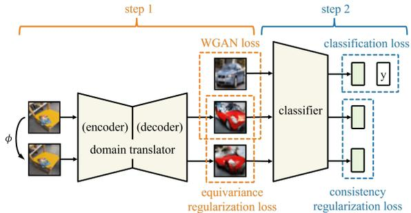
Figure 3. Overview of our two-step algorithm for learning unforeseen robustness from out-of-distribution data. First, we train an equivariant and accurate domain translator using the equivariance regularization loss and the WGAN loss. Second, we use the trained domain translator to translate all out-of-distribution data into target-like ones while preserving the considered variations. We then train a robust model using consistency regularization on the domain-translated data.
