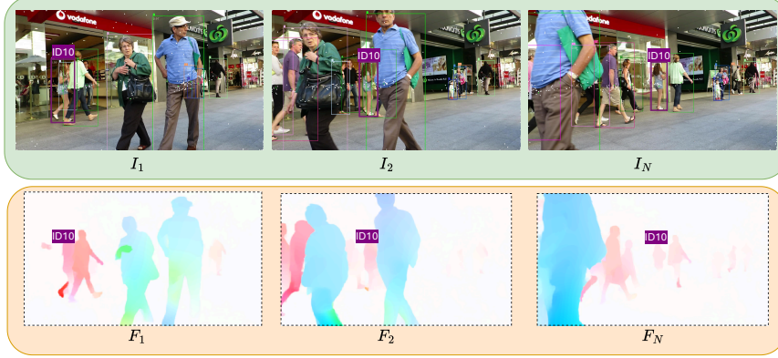
Figure 5. Illustration of MOTE’s capability to track occluded subjects in challenging scenarios using optical flow. The top row shows consecutive frames ( I_1, I_2, \dots, I_N ) from a video sequence, where multiple subjects, including ID10, are partially occluded. The bottom row displays the corresponding flow fields ( F_1, F_2, \dots, F_N ) computed by the optical flow estimator. These flow fields capture the motion between consecutive frames, allowing our method to maintain accurate tracking of occluded subjects by leveraging the motion information. The effectiveness of our approach in handling occlusions is evident from the continuous tracking of ID10 across frames, even when it becomes partially occluded by other subjects. Note how the flow field maintains strong motion cues (shown in color intensity) even in regions of partial occlusion, enabling MOTE to predict object trajectories through occlusion events. The flow visualization uses standard color coding: hue indicates direction and saturation indicates magnitude of motion.
