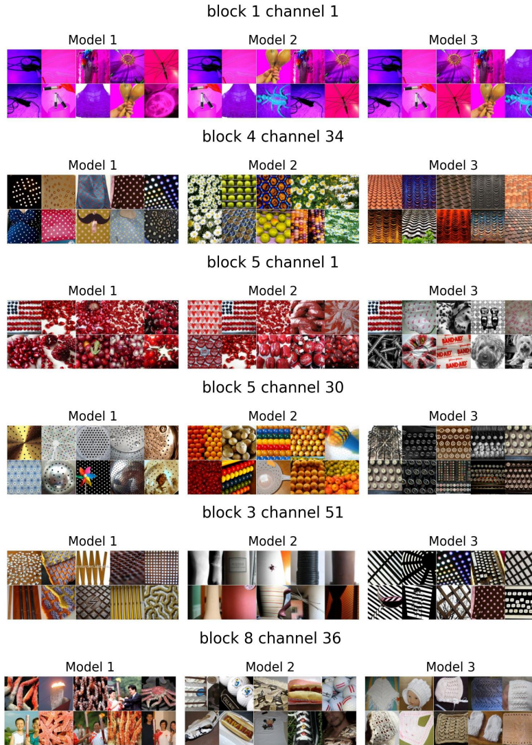
Figure 15: Top activated images from 3 ResNet18 models. Model 2 and 3 are more aligned to model 1 after permutation. In some cases, we have only one model (2 or 3) visually aligned to model 1. There are also cases that neither of the 2 models shows FV similarity after permutation.
