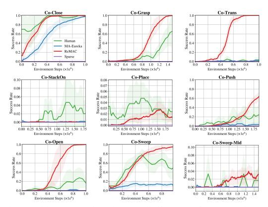
Figure 4: Training curves on various tasks. ReMAC significantly outperforms other baselines and surpasses human-designed rewards in most tasks.
