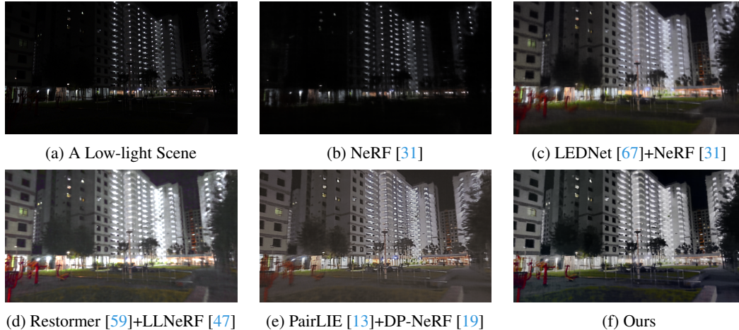
Figure 1: Given a hand-held captured low-light scene (a), while (a combination of) existing low-light enhancement/NeRF methods may not produce visually pleasing novel-view images ((b)-(e)), our LuSh-NeRF can produce bright and sharp results (f).
