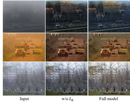
Fig. 6. The impact of brightness loss on dehazing results.
