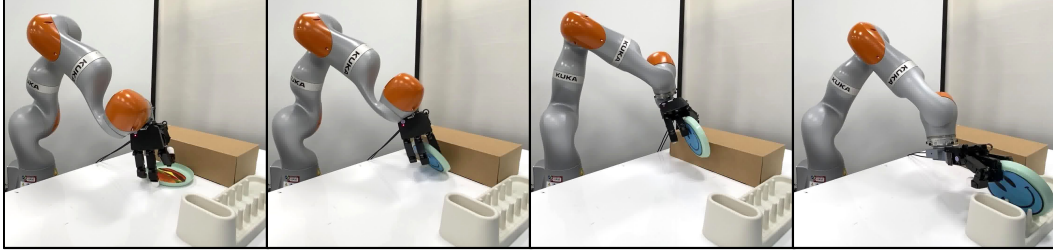
Figure 13: Plate Pivot Lift Rack. Robot converges on a strategy that is guided by the human demonstration, but adapted to its morphological differences.
