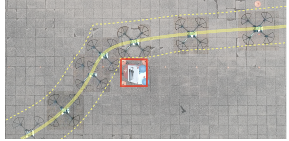
Fig. 1: Timelapse of quadrotor with Exponential Control Barrier Functions (ECBFs) enabled to avoid a virtual obstacle. The quadrotor follows a nominal trajectory toward goal point (orange cone at top right) that would have passed through obstacle without safe control. We use this setup to identify key failure cases of deploying ECBFs in the wild.
