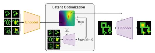
Figure 1: Inference of the Latent Program Network (LPN) model. (Left): the encoder maps I/O pairs to a latent space of encoded programs. (Middle): the latent program is refined during an optimization process to best explain the given I/O pairs (figure detailed in the appendix at Figure 20). (Right): the decoder executes the latent program to generate the desired output for a newly given input.
