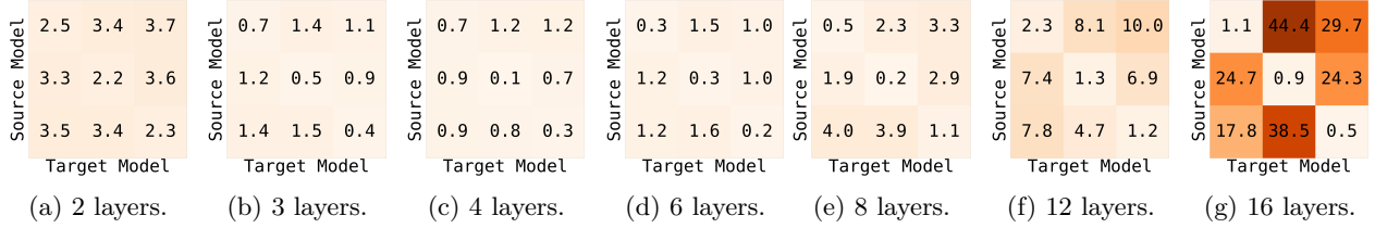
Figure 20: Same as above figure (19) but adversarial samples were generated using label-attack with k = 7 . As with feature-attack , transfer of adversarial samples across transformers progressively becomes poorer as number of layers increases.
