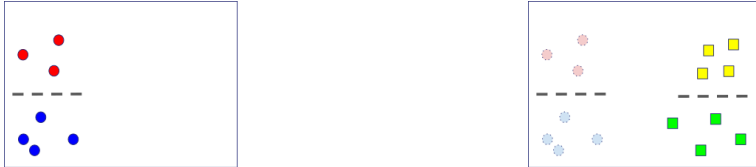
Figure 4: Simple case of continual learning classification in a multi-task setting. Left, the task T_0 : learning a hyperplane splitting two classes (red and blue dots). Right, the task T_1 : learning a line splitting two classes (yellow and green squares) while remembering T_0 models without remembering T_0 data (pale red and blue dots).
