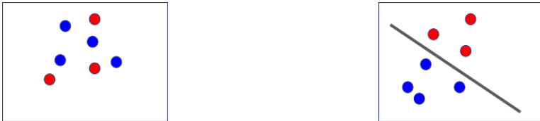
Figure 5: \mathbb{D}_0 feature space before learning T_0 (Left), \mathbb{D}_0 feature space after learning T_0 with a possible decision boundary (Right). Data points are shown by blue and red dots. The line (right part) is the model learned to separate data into the feature space.
