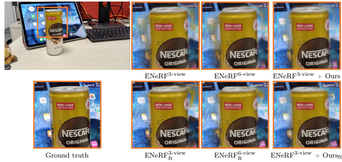
Fig. 7: Visual effects of different ways of combining more input views. Artifacts in disocclusion regions cannot be resolved by including more input views for a single cost volume. Our method could alleviate these artifacts by combining more cost volumes in rendering.
