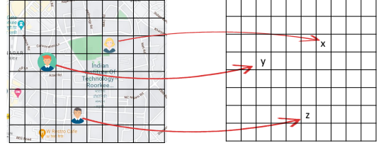
Figure 2: Spatial region with grid for representation as model with (x,y,z) as scalar observations from different participants
