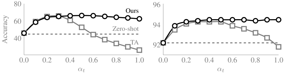
Figure 2: Left: We merge models trained on 8 image classification tasks with a pretrained ViT and vary \alpha_t . Our method performs similarly to TA for smaller but significantly better for higher \alpha_t , improving over the best \alpha_t for TA. Right: We add four sentiment analysis tasks to RoBERTa trained on IMDB. Our merging function dominates TA and requires no tuning of scaling factors. We plot the average over individual dataset accuracies.
