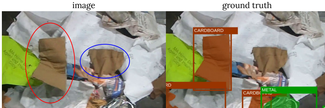
Figure 4: Left: example of an image from ZeroWaste-f dataset. Right: the corresponding ground truth instance segmentation. Expert training and common sense knowledge are required to distinguish between the cardboard object on the left (red circle) and the brown paper on the right (blue circle), as they are visually very similar but differ in thickness and rigidity ( best viewed in color ).
