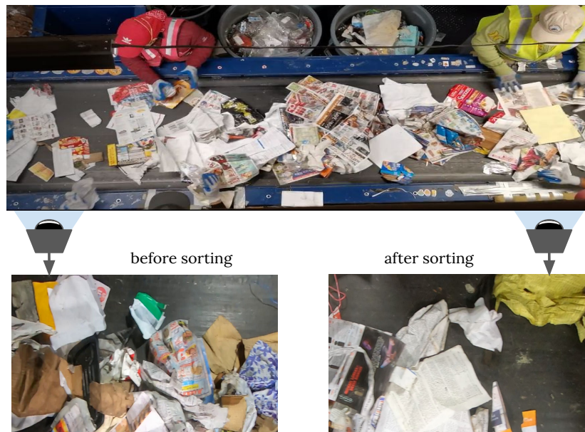
Figure 5: We installed two stationary cameras above the conveyor belt: one at the beginning of the line and another one at the end. At this particular conveyor belt, workers are asked to remove objects of any material other than paper, such as cardboard, plastic and metal. Therefore, the footage collected from the beginning of the line contains the “foreground” objects that need to be removed, and the frames from the end of the conveyor belt are supposed to only contain the “background” paper objects. We used this setup as a foundation of our ZeroWaste-w dataset.
