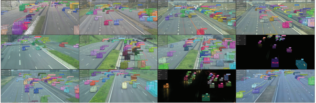
Figure 3. Visualization of the labeled TUMTraF-Accid3nD dataset with 3D box annotations, instance masks, track IDs, and trajectories. Accidents are recorded from roadside cameras on a test bed for autonomous driving. The dataset includes scenes with collisions and overturning vehicles, with some vehicles even catching fire.
