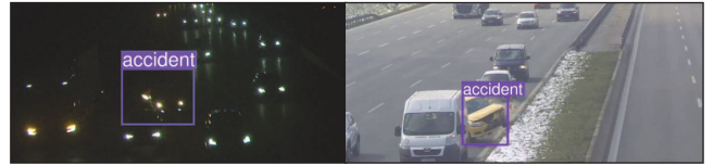
Figure 13. Qualitative results of our accident detection framework on the TUMTraf-Accid3nD test set. Left: The rule-based approach detected a rear-end collision. Right: The learning-based approach detected a car crash with a confidence score of 0.8.
