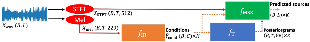
Figure 1: The proposed Jointist framework. This framework can transcribe/separate up to 39 different instruments as defined in Table 11 in the Appendix. B : batch size, L : audio length, C : instrument classes, T : number of time steps, K : number of predicted instruments. The dotted lines represent iterative operations that are repeated K times. Best viewed in color.
