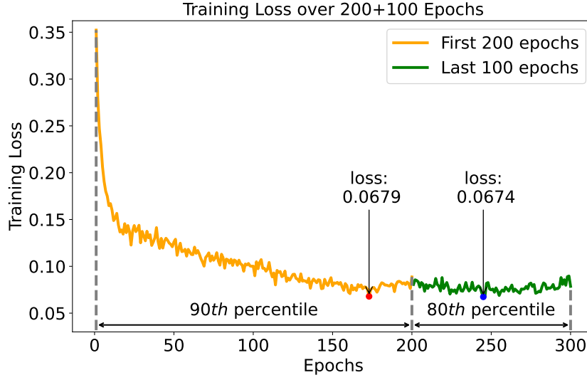
Figure 13: (best in color) Training loss of FoMo-0D ( D = 100 ) with 0.5K unique + 7.5K transformed datasets/epoch for 200 epochs (in orange), followed with additional 100 epochs of training (in green). For the first 200 epochs we train with 90th percentile as the inlier/outlier threshold, which we reduce to 80th in the subsequent 100 epochs.
