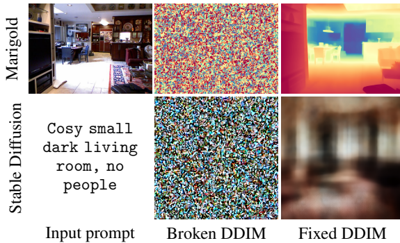
Figure 5: Single-step outputs of Marigold and Stable Diffusion. With a single step, Stable Diffusion produces a blurry image at best, while Marigold outputs a sensible depth map. Note that the input prompt is text for Stable Diffusion, but an RGB image for Marigold.
