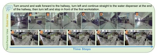
Figure 16: Example of a robot successfully navigating in a real environment without human presence. The figure presents the instruction given to the robot (top), the robot's view captured by the fisheye camera (middle), and a third-person view of the robot's navigation (bottom). [Zoom in to view]
