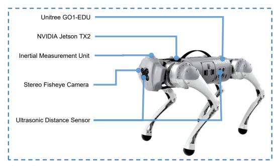
Figure 15: Real-world robot used in our experiments. The robot is Unitree GO1-EDU, a quadruped robot equipped with an NVIDIA Jetson TX2 high-performance computing module for handling computational tasks. The robot features an Inertial Measurement Unit (IMU) for measuring acceleration and rotational speed, a Stereo Fisheye Camera for wide-angle perception of its surroundings, and an Ultrasonic Distance Sensor for measuring the distance between the robot and obstacles.
