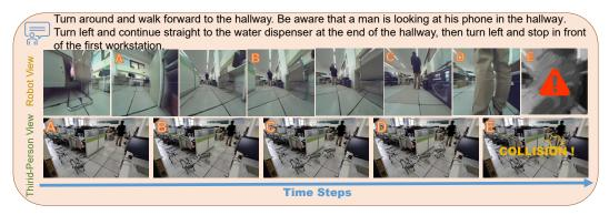
Figure 18: Example of robot navigation failures in real environments with human presence. The robot collides with a human when their status changes unexpectedly, leading to a mission failure. [Zoom in to view]
