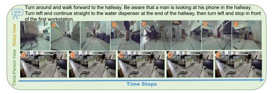
Figure 17: Example of a robot successfully navigating in a real environment with human activity. The robot observes humans, adjusts its path, circumvents them, and reaches its designated destination. [Zoom in to view]
