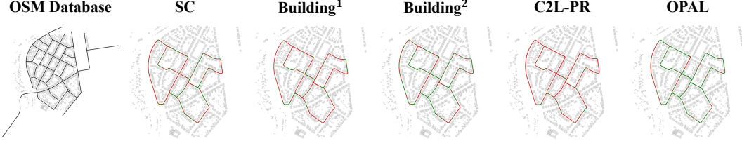
Figure 3: Top-1 retrieved results @5m threshold on the 00 sequence of the KITTI dataset. Black points • denote OSM tile locations, while red • and green • indicate the wrong and correct retrieved results, respectively.
