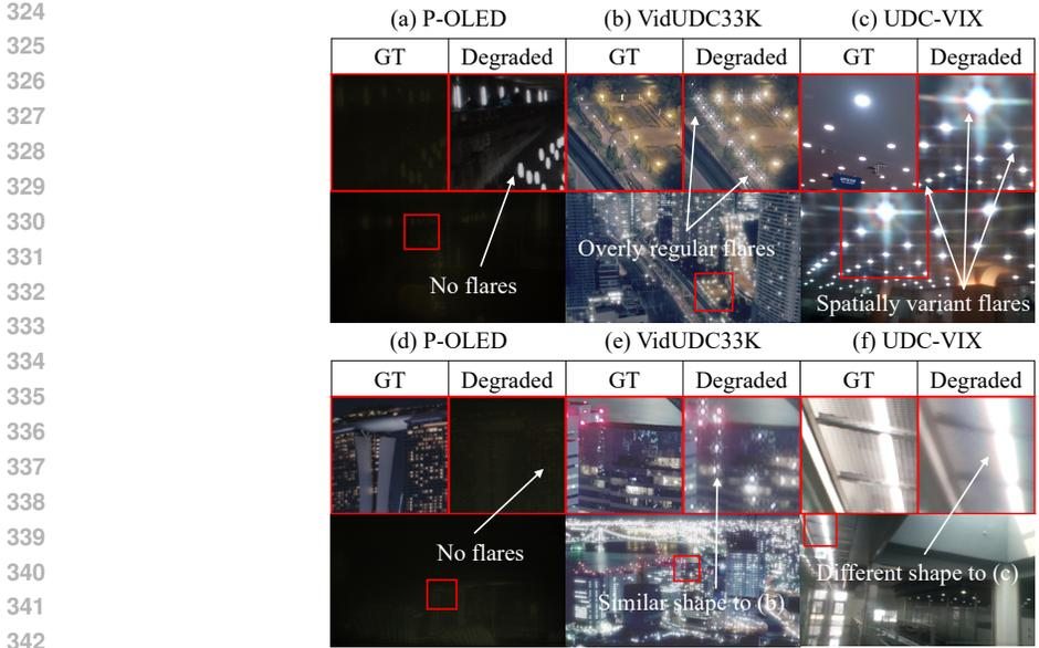
343 Figure 5: Comparison of flares. P-OLED shows no flares ((a) and (d)). VidUDC33K displays overly
