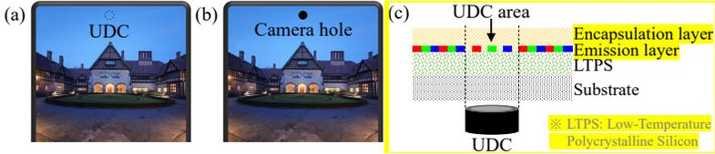
Figure 1: Comparison between under-display (UDC) and traditional hole-display cameras. (a) UDC. (b) Hole display camera. (c) The pixel structure of the UDC area. The UDC area exhibits a reduced pixel density due to the pixel pattern acting as diffraction slits.
