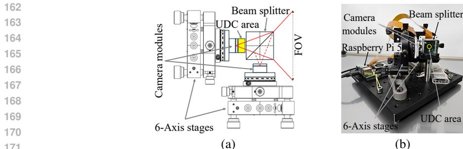
Figure 2: The UDC video-capturing system. (a) The optical layout of the dual camera combiner. The UDC area is enlarged for a better view. (b) The proposed video-capturing system.
