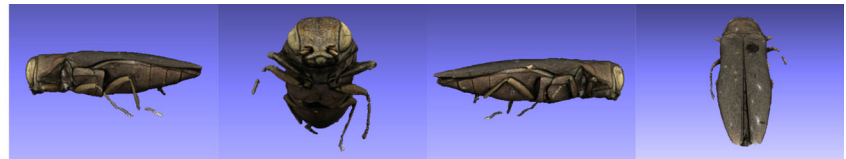
(a) Moving lens & stacking with SIFT feature based homography (MHD = 0.003072)
