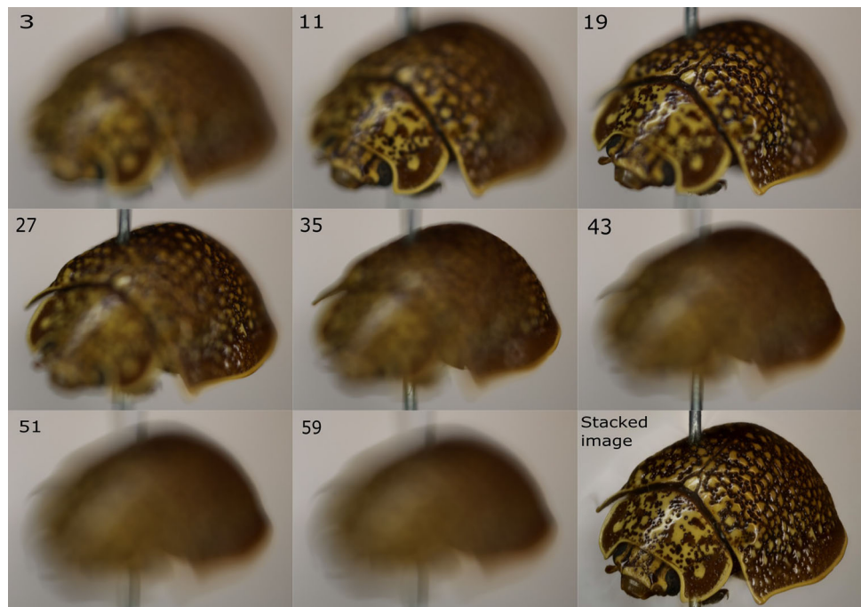
Fig. 3 A set of 61 partially out-of-focus images (only eight of them shown here) captured at different camera positions are stacked to produce an in-focus image. The stacked image, however, does not represent a single perspective image formation due to the moving lens. (Best viewed in colour on the screen)
