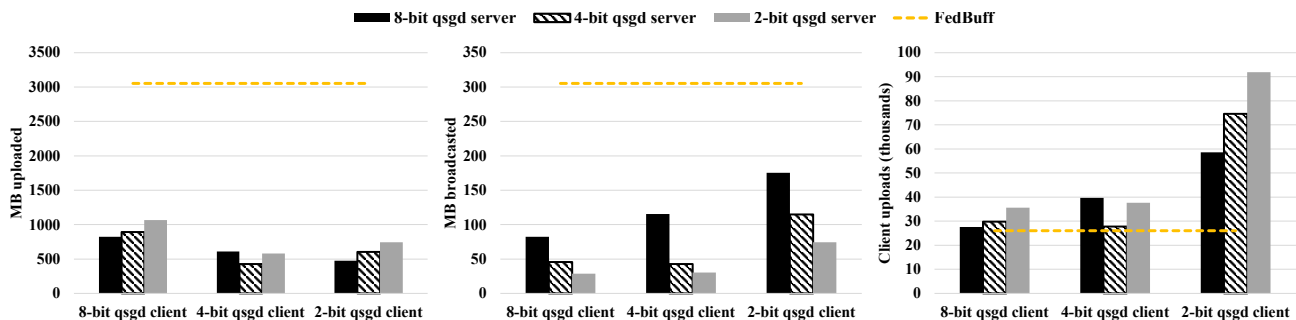
Figure 4. Communication metrics of QAFel and FedBuff to reach target validation accuracy (90%) with varying choices of qsgd quantizers. In all cases QAFel saves at least 3\times upload cost and 2\times broadcast cost. Notice that in 4-bit qsgd client and server, the convergence speed is the same for both algorithms, and the upload message size goes down from 3052 MB to 428 MB, a 7\times decrease, with analogous decrease in download cost.
