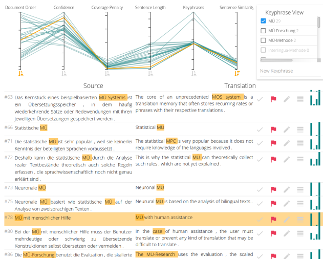
Figure 4: Main view of the system: the Document View shows some flagged sentences for correction. Additionally, the keyphrase filter (top right) is active: all sentences containing the keyphrase ‘MÜ’ are shown in the Metrics and Document Views. It is visible that ‘MÜ’ is never correctly translated to ‘MT’.
