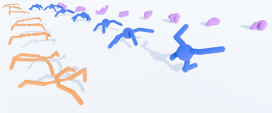
Figure 1: Diverse motion behaviors and robot morphologies generated by RoboMoRe. Orange: A bio-inspired long-legged robot crawling forward in a climber posture. Blue: A uniform robot advancing by jumping. Purple: A low-center-of-gravity robot rolling forward along the ground.
