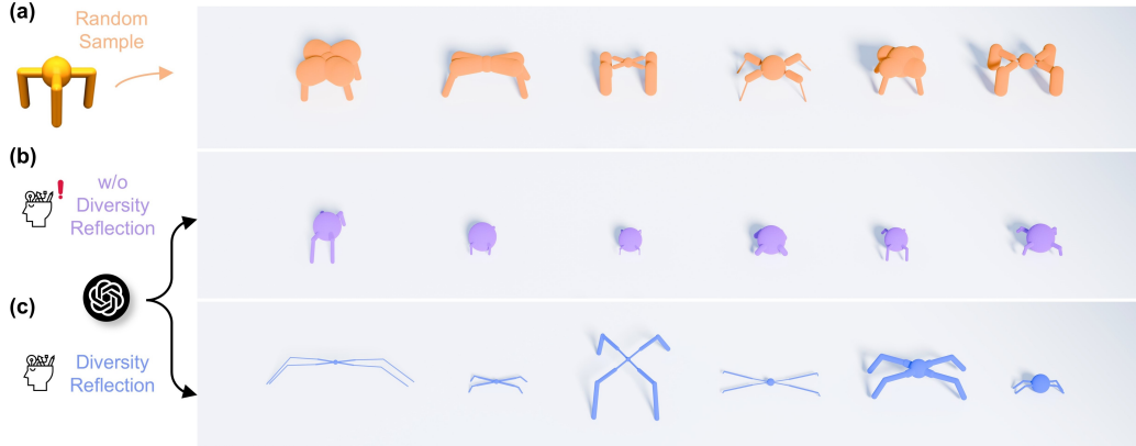
Figure 6: Qualitative results among (a) Random Sample, (b) RoboMoRe (w/o Diversity Reflection), (c) RoboMoRe. It can be observed that RoboMoRe with Diversity Reflection could generate more high-quality and diverse robot morphology examples compared to others.
