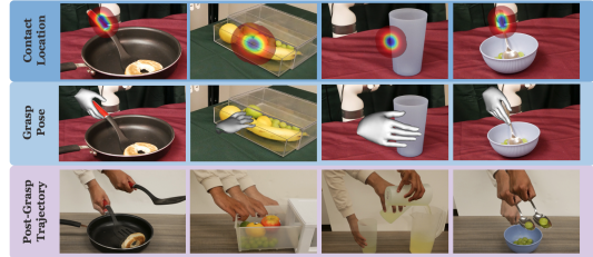
Figure 3: We produce three priors from human videos: the contact location ( top row ) and grasp pose ( middle row ) from the affordance prior; the post-grasp trajectory ( bottom row ) from a human demonstration of the task.
