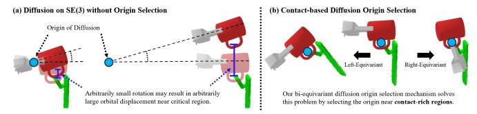
Figure 3. **Necessity of Diffusion Origin Selection Mechanism.** (a) A small rotational diffusion may result in arbitrarily large orbital displacement near the critical region depending on the diffusion origin. (b) We employ a contact-based diffusion origin selection mechanism. This not only allows bi-equivariant diffusion process but also stabilizes learning by minimizing the orbital impact of the rigid body rotation near the critical regions.
