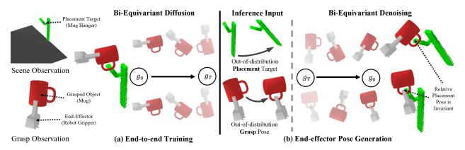
Figure 1. Overview of Diffusion-EDFs. (a) The target end-effector pose  $g_0$  is bi-equivariantly diffused for the training of Diffusion-EDFs. (b) The end-effector pose is sampled from the policy by denoising with learned bi-equivariant score function. Due to the bi-equivariance, the trained policy can be effectively generalized to previously unseen configurations in the observation of the scene and the grasp.
