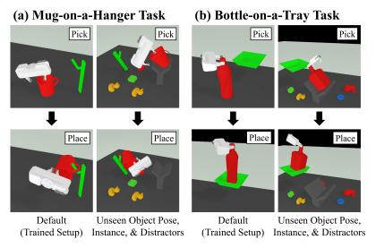
Figure 7. **Simulation Experiments.** (a) In the *Mug-on-a-Hanger* task, a red mug should be picked up by its rim and placed on a green hanger by its handle. (b) In the *Bottle-on-a-Tray* task, a red bottle should be picked up by its cap and placed on a green tray.
