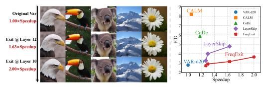
Figure 1: We introduce **FreqExit**, a dynamic inference strategy for next-scale visual autoregressive generation with a proposed frequency-aware guidance, bridging the gap between step-wise generation and early-exit-based acceleration. It achieves up to  $2 \times$  **speedup** with negligible quality degradation, offering a superior trade-off between efficiency and fidelity compared to prior baselines.
