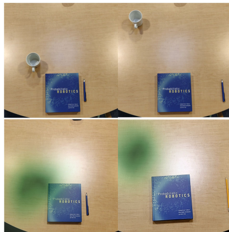
Fig. 6: A small real-world demo. We visualise the learned cost function for placing a mug in a desirable way.
