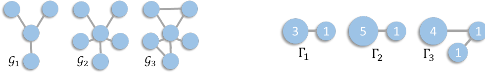
(a) The graph \mathcal{G}_1 has four nodes and three edges. In \mathcal{G}_2 , the graph gains two more nodes and two edges. However, only in \mathcal{G}_3 do two triangular edges emerge in the graph. (b) Induced TDA Mapper networks \Gamma_1, \Gamma_2 and \Gamma_3 for \mathcal{G}_1, \mathcal{G}_2 and \mathcal{G}_3 by using degree as the node feature. Mapper node sizes (denoted by numbers) indicate cluster sizes.
