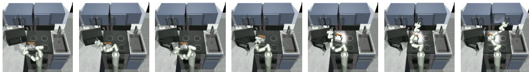
Figure 3: Example demonstration observations. In this [microwave,kettle,switch,slide] task demonstration, the robot first opens the microwave, then moves the kettle to the back burner, turns on the light switch, and finally opens the sliding cabinet.
