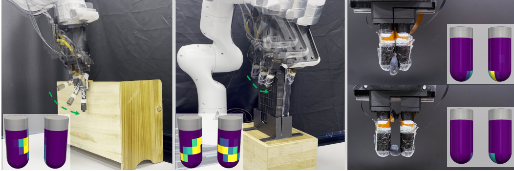
Figure 1: DexSkin sensors enable contact-rich robotic manipulation policies. We demonstrate the applications of DexSkin in in-hand pen reorientation, box packaging, and berry transporting tasks. In each frame, we visualize tactile readings from DexSkin as heatmaps, where brighter readings correspond to larger forces. DexSkin’s high-coverage sensing capabilities enable it to provide contact signals for a variety of robotic manipulation tasks. At the same time, it possesses desirable properties for learning-based manipulation systems.
