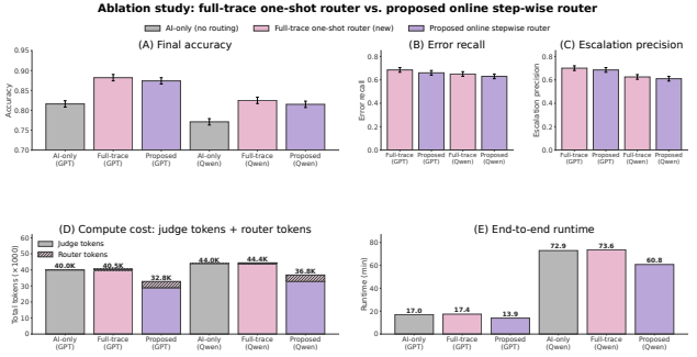
Figure 5. Ablation study: online stepwise monitoring versus full-trace one-shot routing. (A) Final accuracy, (B) error recall, (C) escalation precision, (D) total tokens, and (E) end-to-end runtime.
