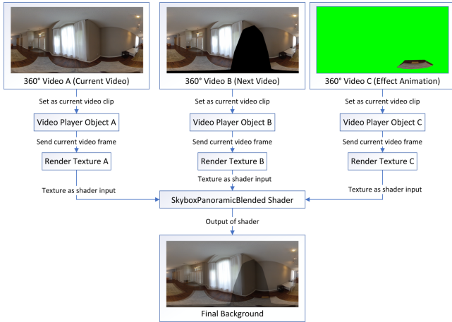
Figure 4: The Video Manager render pipeline, illustrating the high-level process of how the 360 VR environment is made.
