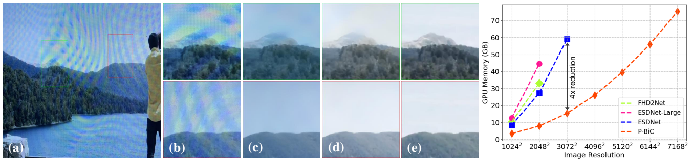
Figure 1: Left: Examples of ultra-high-definition image demoiréing. (a)-(b) The degraded image with a resolution of 3840 \times 2160 from the UHDM dataset [46]. (c) Results generated by ESDNet-L [46]. (d) Results generated by our proposed P-BiC. (e) Ground-truth images. The presented results effectively highlight the superior capability of P-BiC in eliminating undesired moiré patterns and preserving intricate textures. Right: Comparison of GPU memory utilization among distinct image demoiréing techniques. Missing data points indicate that moiré images at these resolutions cannot be reconstructed on an 80GB GPU (NVIDIA A100) due to memory limitations. P-BiC stands out by not only restoring moiré images up to a resolution of 7168 \times 7168 , but also achieving a remarkable 4-fold reduction in memory utilization when restoring an image of 3072 \times 3072 , as compared to the method presented in [46]. Notably, these values are derived from feeding the entire image into the GPU for demoiréing.
