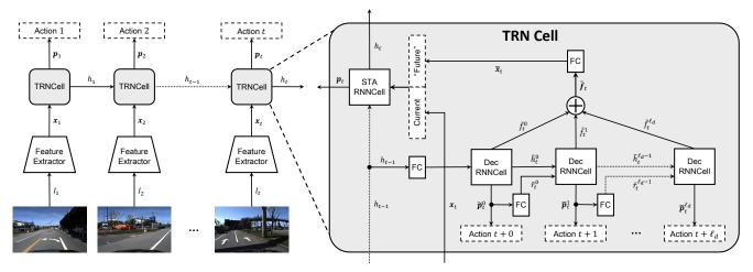
Figure 2: Our proposed Temporal Recurrent Network (TRN), which sequentially processes input video frames and outputs frame-level action class probabilities, like any RNN. But while RNNs only model historical temporal dependencies, TRN anticipates the future via a temporal decoder, and incorporates that predicted information to improve online action detection.
