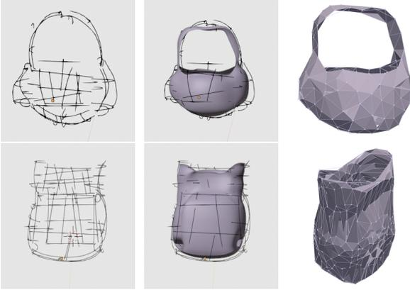
Figure 8. Different 3D models created from real-time 3D sketches with our Blender frontend.
