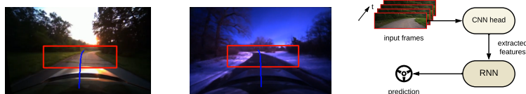
Figure 8: Lane-Keeping task. The first two figures show summer and winter conditions, respectively. The red rectangle indicates the input and the blue line the predicted steering angle of the network. The third figure illustrates the overall network architecture for this task. The CNN head extracts the input features of a video stream. They are passed to the recurrent policy, responsible for steering.
