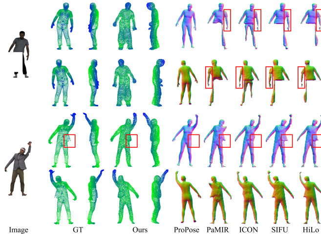
Figure 4: Qualitative results on CAPE dataset. We evaluate our method with SMPL estimation method and implicit-function-based methods. Given the upper image, PaMIR, ICON, and HiLo cannot generate the occluded regions. They cannot also handle the misaligned SMPL mesh on the arms, creating incomplete bodies. ProPose predicts the full-body shape, but cannot capture the details like the blazer of the lower image. However, MHCDIFF is robust to the occlusion and misalignment, and can capture pixel-aligned details.
