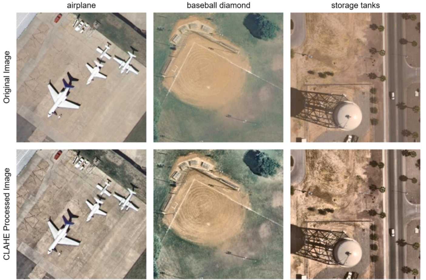
Fig. 5. Sample preview of the original and CLAHE-processed images from three different land use classes in the UC Merced Land Use Dataset. The top row includes the original images for the following classes: airplane, baseball diamond, and storage tanks. The bottom row shows the CLAHE-processed images for the same classes.
