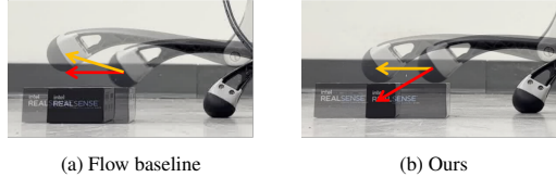
Figure 9: Low-level Control Error. Red arrows denote commanded movements, yellow arrows represent actual movements.
