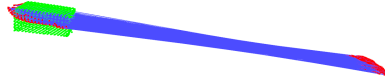
Figure 11: Registration Error: The red point cloud on the right represents the captured object, while the green point cloud indicates the target object pose. The registration result mistakenly shows the object as flipped.
