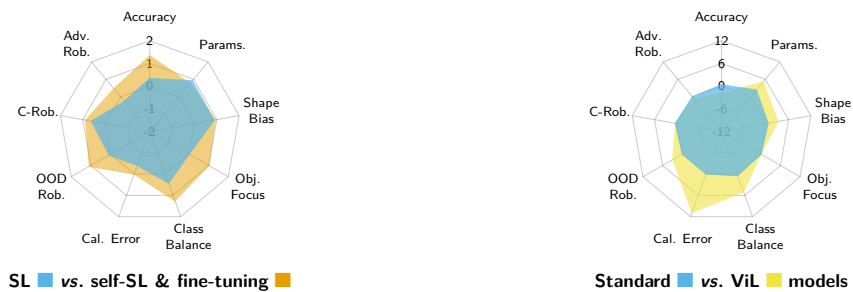
Figure 1: Visualization of two of our main results. We compare nine different quality dimensions for popular backbone models trained with standard supervised learning ■ (SL) against the corresponding backbones trained after initialization with weights obtained through self-supervised learning ■ ( left ) and when utilized in a vision-language (ViL) model ■ ( right ). Axis units indicate the distance (in standard deviations) to the mean (0 line) of each quality dimension; see Eq. (1) and its explanation for details. Please refer to Tab. 2 (e) and (j) for raw values and Sec. 3 for an interpretation of the results.
