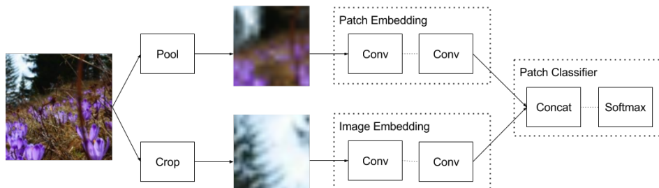
Figure 1: Starting from a high-resolution image (far left), our model creates a low-resolution version through average pooling and a high-resolution patch by taking a random crop of the original image. Each of these two new images is embedding by a series of convolutions and the embeddings are concatenated and fed to a patch classifier. The classifier must predict whether the patch belongs to the image (negatives are created by sampling patches from other images in the batch). We also trained a regression variant which must instead predict the coordinates of where the patch was cropped (not shown).
