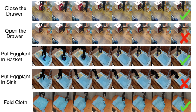
Fig. 11. Samples of autonomous policy evaluation trials with AutoEval on the five tasks. The classifier result of each task is visualized on the right hand side, and the reset policy is not shown.
