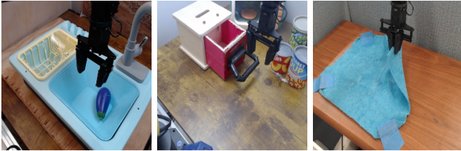
Fig. 3. Five autonomous evaluation tasks across three scenes: two pick-and-place tasks in sink , two articulate object manipulation tasks in drawer , and one deformable object manipulation task in cloth .
