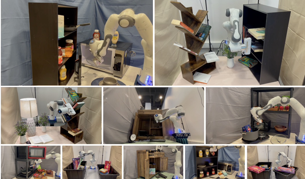
Figure 1: Neural Motion Planning at Scale in the Real World Our approach enables a single, generalist neural network policy to solve motion planning problems across diverse setups; Neural MP can generate collision free motions for a wide array of unseen tasks significantly faster and with higher success than traditional as well as learning-based motion planning approaches.
