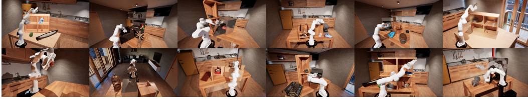
Figure 2: Visualization of Diverse Simulation Training Environments: We train Neural MP on a wide array of motion planning problems generated in simulation, with significant pose, procedural asset, and mesh configuration randomization to enable generalization.
