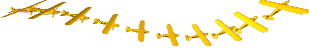
(a) Expert demonstration of a high angle-of-attack perching maneuver that minimizes velocity at the goal position with complex, post-stall aerodynamic forces.
