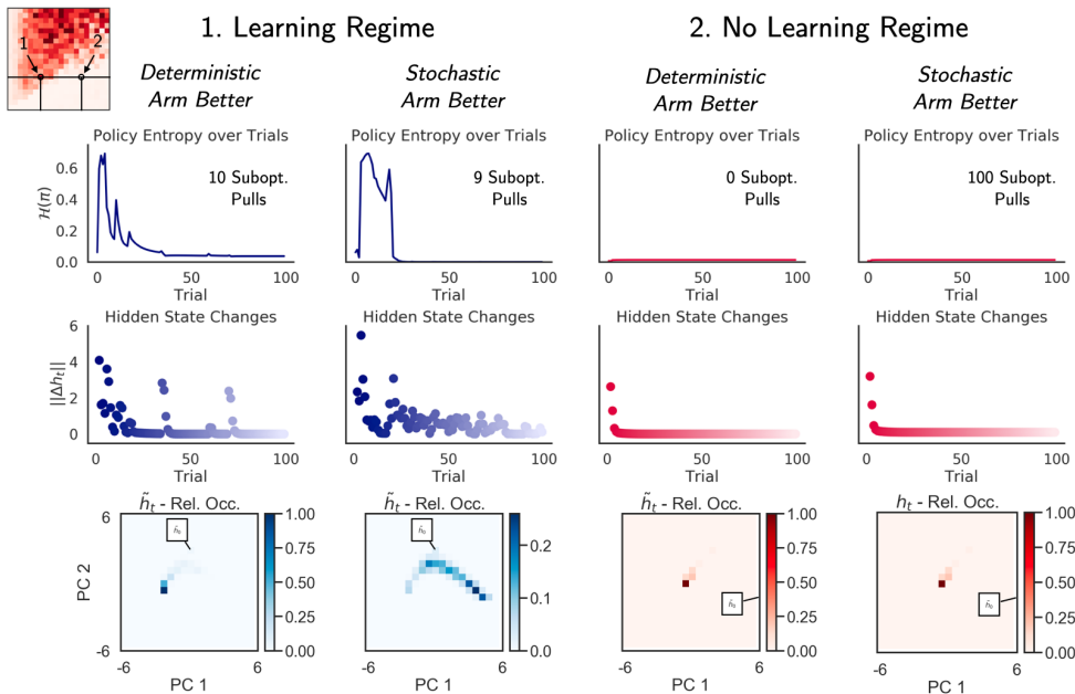
Figure 3: Recurrent dynamics of two meta-trained bandits for task conditions that favour learning (blue) and not learning (red), for a lifetime T = 100 . Each bandit is tested both for the case where the deterministic arm is the better option and for the case where the stochastic arm is the better option. First two columns. Bandit for which an adaptive strategy is predicted by the theory. The inner loop dynamics integrate information which is reflected by the convergence of the hidden state to two different fixed points depending on which arm is optimal. Last two columns. Bandit for which the heuristic choice of the deterministic arm is the Bayes optimal behavior. Not learning manifests itself in non-exploratory, rigid behavior and activations. The final row visualizes the PCA-dimensionality reduced hidden state dynamics ( \tilde{h}_t ) averaged over 100 episodes. A darker color indicates a more frequent occupancy in the discretized PCA space of the transformed hidden states.
